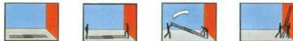
Lay the ladder on the ground with the base at the spot where it is to stand.
